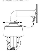
4. Fix two screws to the holes as indicated by the arrows (left) and leave 12mm clearance.
